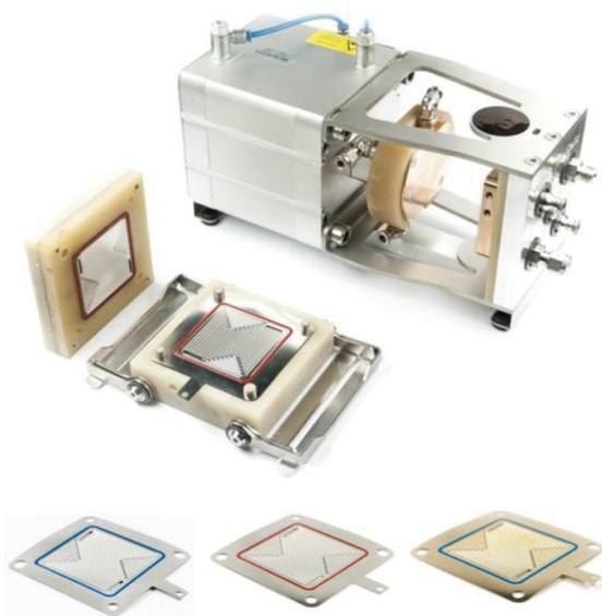
Fig. 3 | A measuring cell from *balticFuelCells* (type quickConnect) modified for the mounting of metallic bipolar plates ([www.zbt-duisburg.de](http://www.zbt-duisburg.de))
